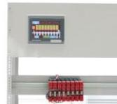
The Pixsys Extrusion Kit is designed to monitor and control extruders, with a maximum number of 8 zones. The application has been developed for the HMI panel mod. TD700, and for the DRR450 controller via the RS485 connection with RTU Modbus communication protocol.
